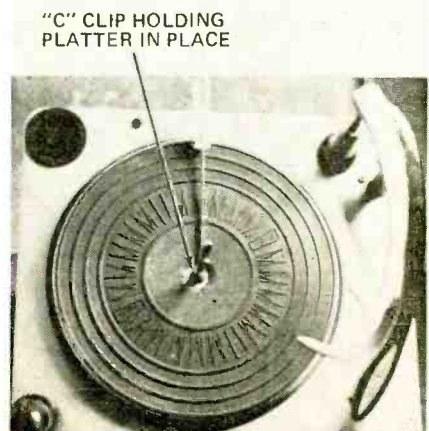
FIG. 1—TYPICAL RECORD CHANGER. Note that there is usually only a single C-clip holding the platter in place.
