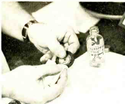
FIG. 4—CLEAN IDLER AND DRIVE wheels thoroughly. Dry with a separate piece of clean towelling.
